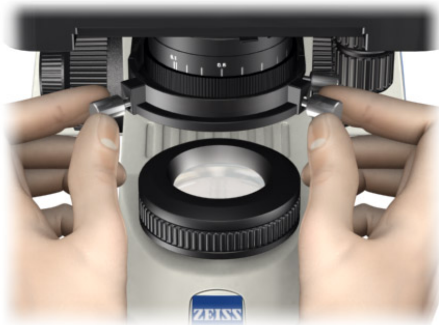
Alignment of the Condenser Along the Microscope Optical Axis
