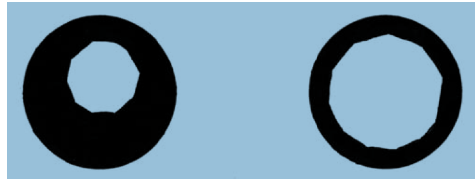
Alignment of the Condenser Along the Microscope Optical Axis
